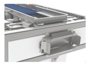
Servo-controlled linear actuators provide maximum flexibility for the realization of different stacking schemes and reduce the effort for the format change to almost a push of a single button. Reliability and fault-free operation are the criteria by which this cartonizer is designed and build. This is also reflected in the used control system of the latest generation.
