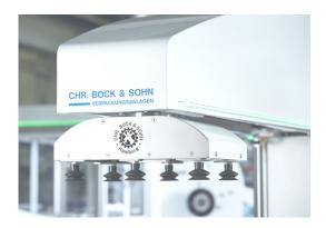
Servo driven linear actuators of the latest generation, controlled via a user friendly touchscreen panel make this palletizer a highly efficient tool for your daily production. Within minutes even a non skilled operator is able to generate completely different packing schemes for a pallet by using the integrated packscheme generator. As the control system permanently stores the current status of the pallet, the palletizer is able to continue its work after an interruption of any kind.
