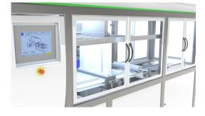
In combination with the CHR. BOCK & SOHN developed volumetrically controlled double piston system DKD, the BPM 2000 achieves an optimum packaging quality and presentation of your product. Our plants are equipped with the latest touch screens and matching controls. This allows an easy and intuitive operation of all recipes and production parameters. With the ,Beluga Clean Line' design, developed by us, in combination with the ,Mood-line' status function a maximum efficiency is always granted.
